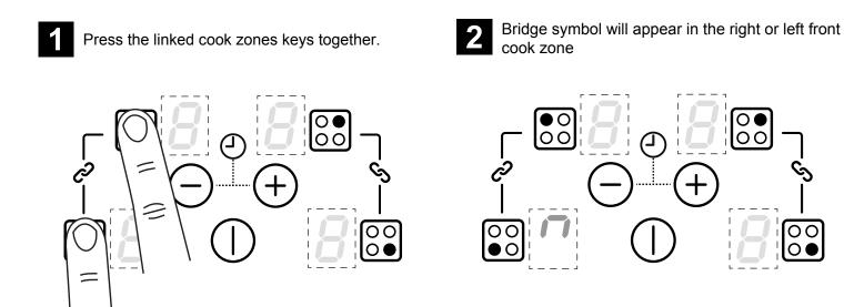
The cooking zones can be used as four separate cooking zones which can be controlled individually. Or, the two left hand zones and the two right hand zones can be bridged to provide two large zones that can be controlled via one setting.
